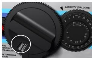
*Fig. 18. Rotate the knob to “brine refill” position*
