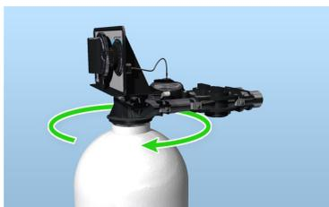
*Fig. 5. While screwing the valve onto the resin tank, make sure the distributor tube locks into place.*
